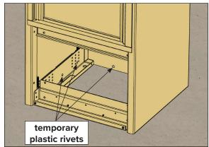
**E.** Remove the two mounting brackets and two skirt plates from the cabinet, and set them aside for later installation.
