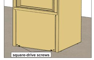
2). Pull the panel out at the bottom and down from behind the PORT package-box trim.
